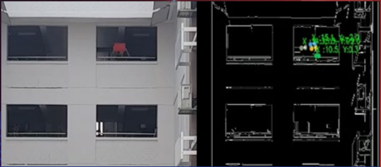
Figure 9: HTX conducting a test to ascertain that TILDE could detect distant movements.
