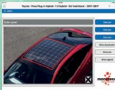
Current generation Prius glass roof extrication hazard (Moditech screen shot).
