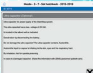
Stop/start ultra-capacitor hazards (Moditech screen shot).
