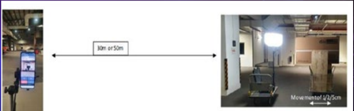
Figure 11: The setup of a night trial to simulate night operation conditions.
