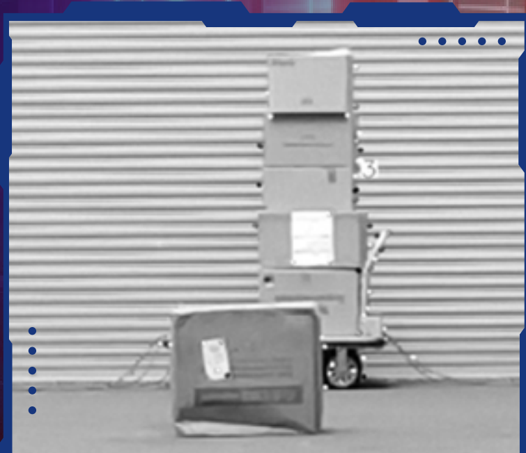
Figure 10: TILDE was able to detect 1cm movement from 30m away, and 2cm movement from 50m away. The white dots indicate the corners that are detected by TILDE.
