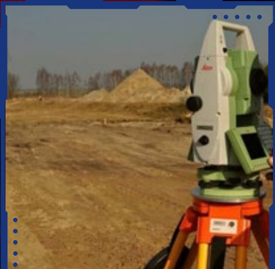
Figure 2: Image of a total station. Users view an object from a distance through the lens of the total station. With the marking on the lens, the user can determine if the object has shifted.
