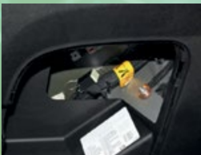
2017 Chevrolet Volt 12V battery emergency responder disconnect area.
