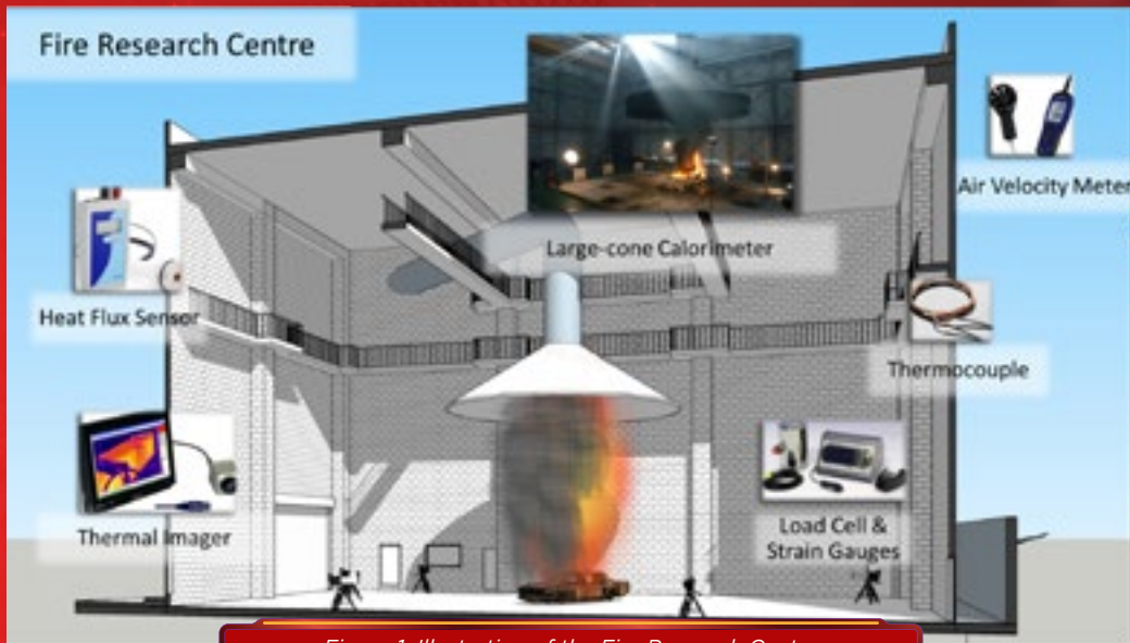
Figure 1: Illustration of the Fire Research Centre facility and its capabilities
