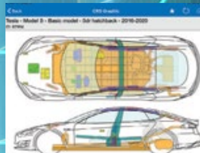
Tesla Model S vehicle floor/battery pack lifting/dash displacement hazard (Moditech screen shot).
