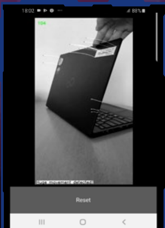
Figure 7: An image showing the user interface of TILDE. Observe how the points around the white label are selected for tracking. The white lines are the path travelled by the tracked points.
