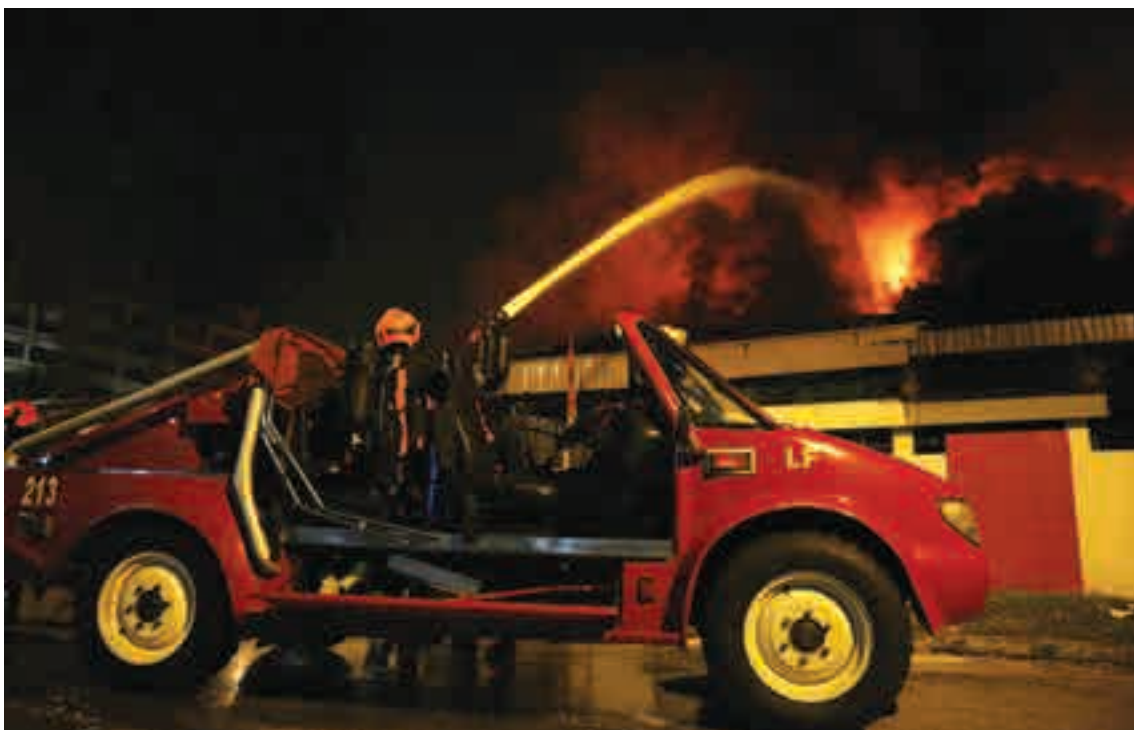
Figure 4: The water monitor of the LFAV being put in action during an industrial fire.
