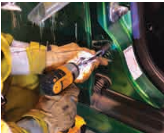
Figure 5: Using an Impact wrench to remove doors and the hinges.
