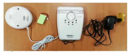
Strobe light with standby battery and vibration device
