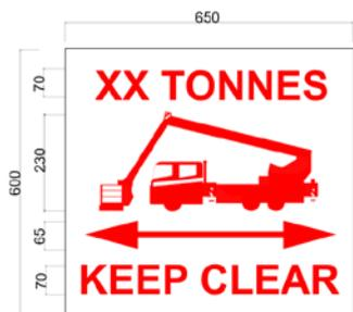
Pictogram to be located at the junction and along the fire engine accessway facing travel direction of fire engine
