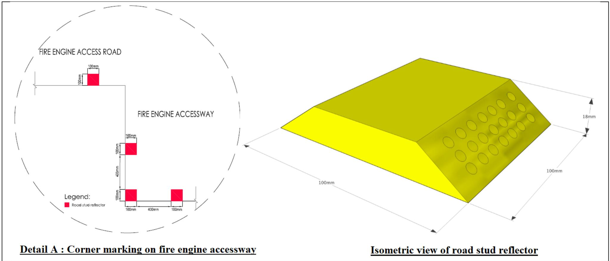
**Pictogram of fire engine access road for firefighting appliance not exceeding 24 tonnes**
