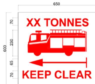
Pictogram to be located at the start or end of fire engine access road, depending on the direction of the fire engine access road
