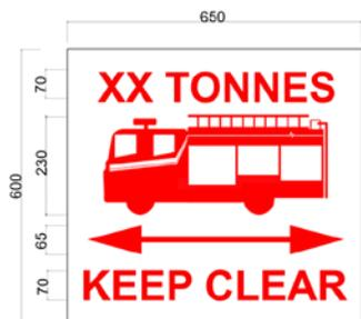
Pictogram to be located at the junction and along the fire engine access road (if any) facing travel direction of fire engine
