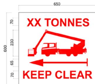
Pictogram to be located at the start or end of fire engine accessway, depending on the direction of the fire engine accessway
