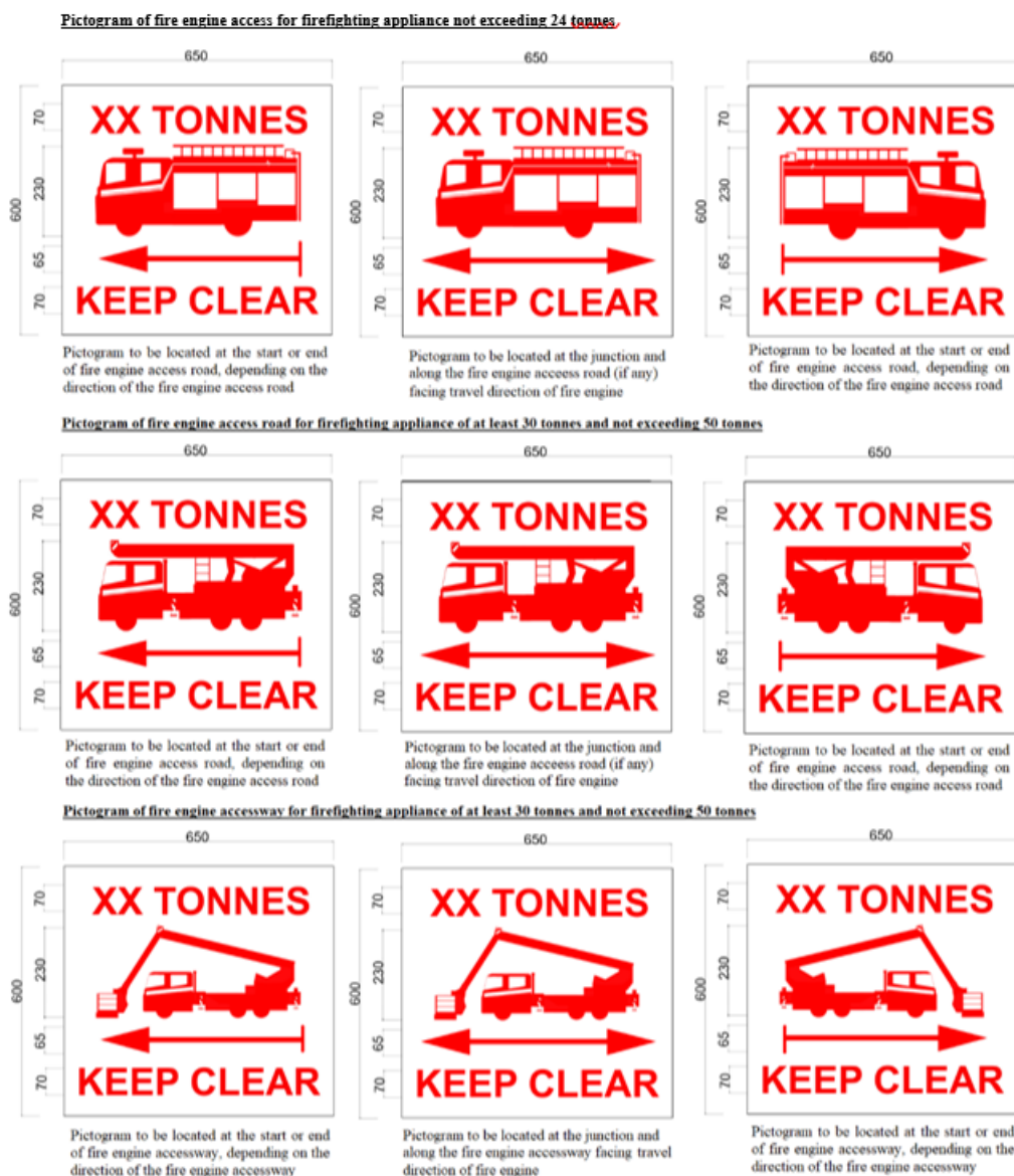
Diagram 4.2.4j.(3): Pictogram signage for Fire Engine Accessway/ Fire Engine Access
