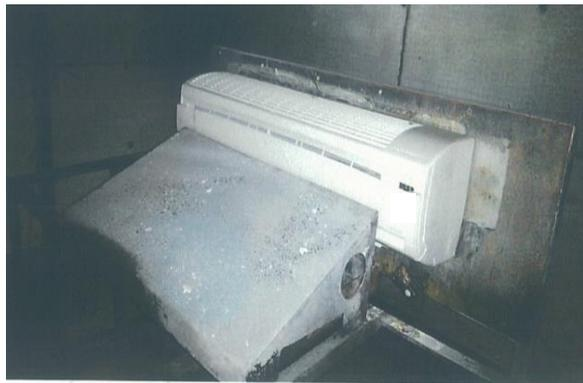
(a) FCU burn test set-up
