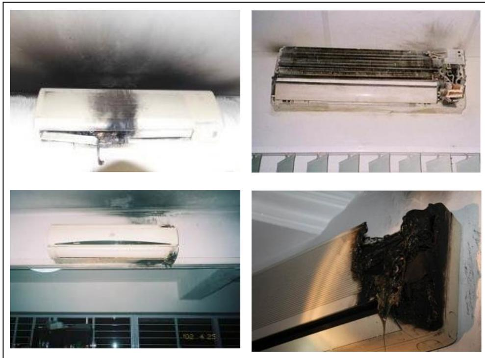
**Figure 13. Localised fires involving FCUs which were on standby mode**
