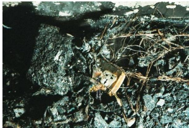
**Figure 15. The burned remains of a portable socket outlet**
