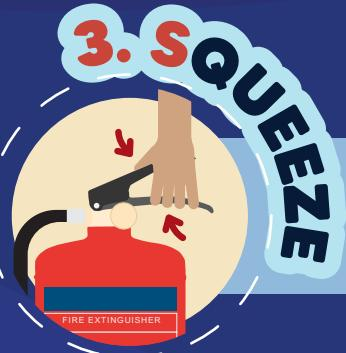
**SQUEEZE** the top lever of the fire extinguisher
