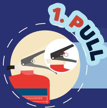
**PULL** out the safety device of the fire extinguisher
