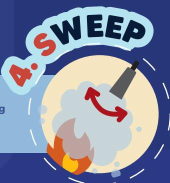
**SWEEP** the nozzle from side to side while directing the discharge at the base of the fire
