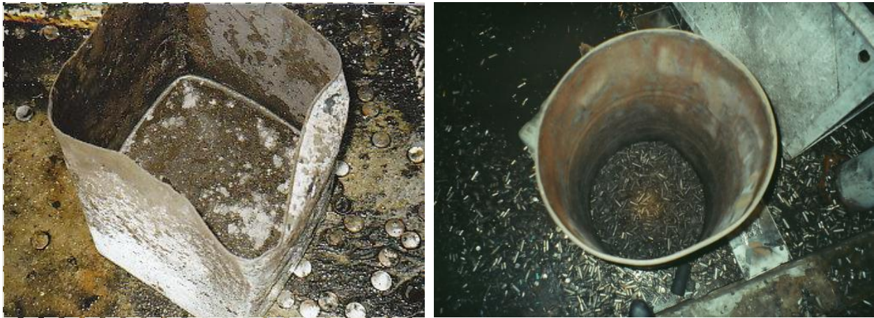
Figure 18. Discarded batteries of various sizes stored in metal containers were involved in fires
