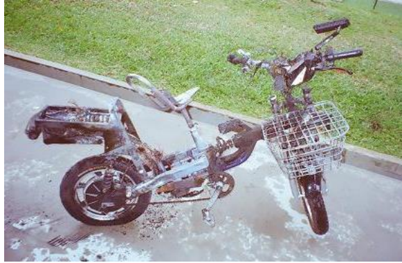
Figure 3. Battery positioned above the rear wheel
