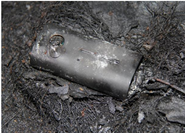
Figure 23. Burnt remains of the powerbank were recovered from the determined Area of Fire Origin
