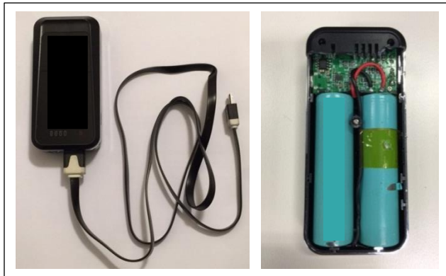
Figure 9. A powerbank with built-in cylindrical Li-ion batteries
