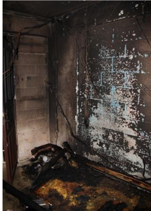
Figure 17. The burn patterns were consistent with fire origin near the main door where the battery of an electric bicycle was being charged.
