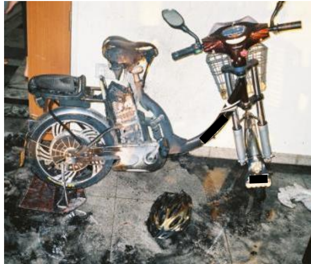
Figure 15. The seat and battery compartment of the electric bicycle were damaged
