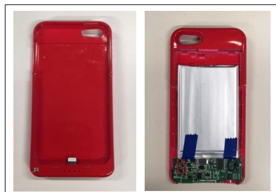
Figure 11. A power sleeve for handphones with a built-in pouch type Li-ion battery
