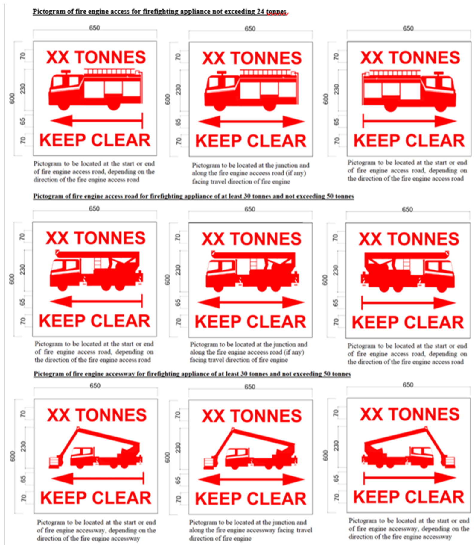
Diagram 4.2.4j(3): Pictogram signage for Fire Engine Accessway/ Fire Engine Access Road
