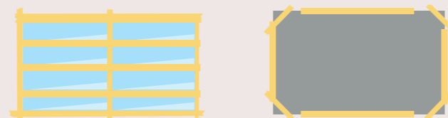
Examples of how the louvred windows can be sealed. The sealing process can be carried out using plastic sheets and tape or by taping over the gaps securely.
