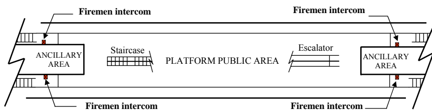
Locations of firemen intercom at platform level
