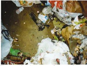
Figure 13. A ruptured aerosol can recovered amongst the refuse
